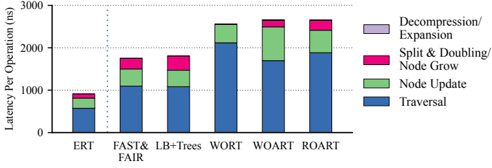
Fig. 1. Latency breakdown for insert operations on several state-of-the-art tree-based PM indexes [18, 22, 29, 32] and our design ERT. We use the Facebook user ID data set.
