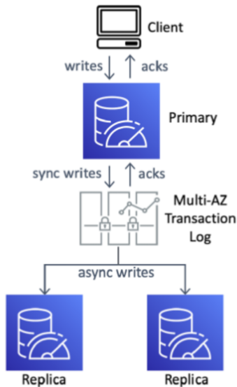
Figure 1: MemoryDB high-level overview. A primary node synchronously executes and replicates updates to a MultiAZ transaction log. Secondary nodes asynchronously fetch updates from the transaction log.
