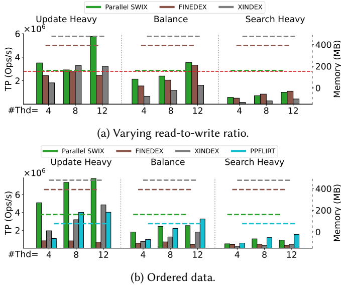
Fig. 14. Comparison of parallel learned indexes on different workloads. Bars represent throughput (TP, left y-axis), while the dashed line indicates memory usage in MB (right y-axis).
