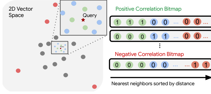
Fig. 8. Illustration of the filter generator methodology. A Positive Correlation workload is then generated by preferentially sampling vectors from the closest neighbors, conversely, for the Negative Correlation.
