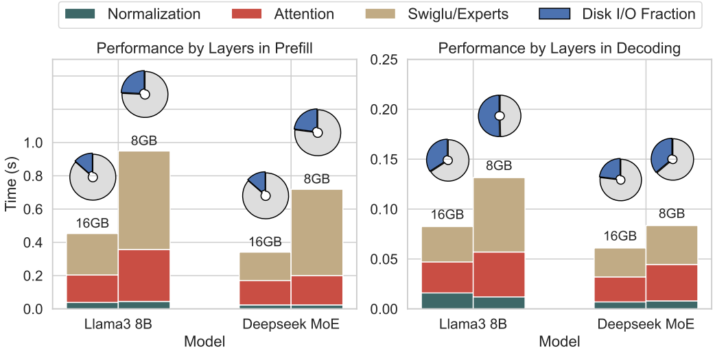
Fig. 12. Layer-wise runtime and disk-I/O fraction for 25-token prompts under varying memory. Prefill performance degrades with less memory (nearly 2× disk I/O). MoE decoding scales better since only a subset of experts is active, reducing I/O.
